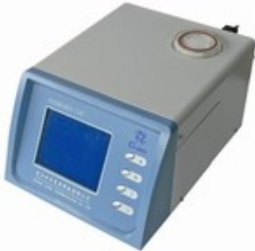
**GASBOARD 5020** is an analyser for the control of exhaust gases from gasoline or LPG engines; it integrates non dispersive infrared (NDIR) detectors for the measure of CO, CO<sub>2</sub>, HC and electrochemical sensors (ECD) for O<sub>2</sub> and NO.
